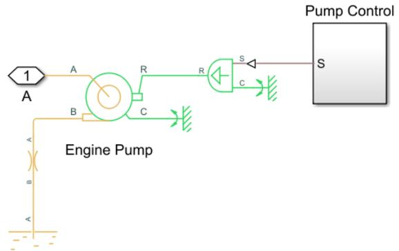
Figure 7. Engine pump and its subcomponents.
