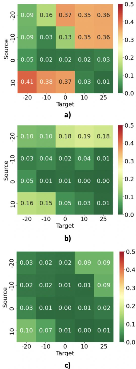
Figure 3. Heatmap of Target Mean Squared Error (MSE) for Different Domain Adaptation Methods under Different Source and Target Temperatures ( $^{\circ}\text{C}$ ). **a)** No TL, **b)** CORAL, and **c)** DARE-GRAM.
