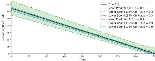
Figure 3. LSTM RUL prediction for testing engine #13 with dropout probability value of 0.3 and 0.9.
