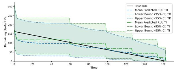
Figure 2. HMM RUL prediction for testing engine #13.
