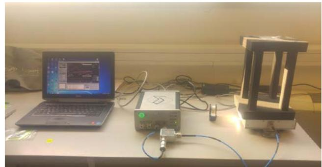
Figure 13. Tagformance®'s test bench for UHF RFID tag characterization
