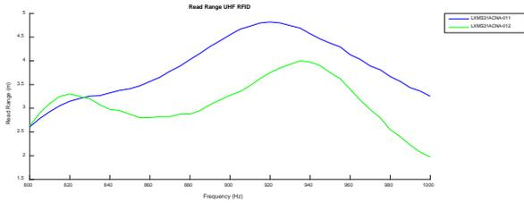
Figure 14. Read range measurements from Meander reference tags obtained with the test bench
