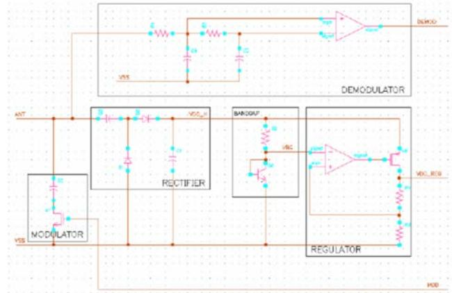
Fig. 10 - Block Diagram of the RF front end
