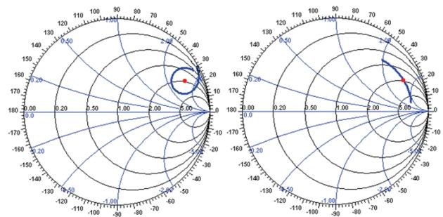
Figure 8. Broad-banded (left) and narrow-banded impedance (right) match between the antenna and the microchip.
