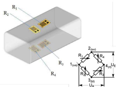
Figure 4. Strain gauge bridge
