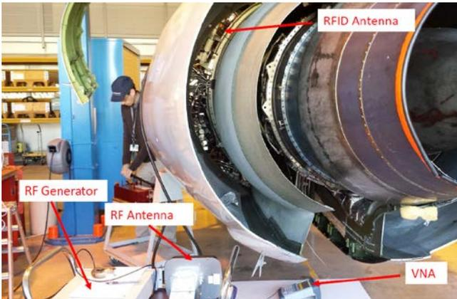
Figure 19. System tests in application environment for the first test
