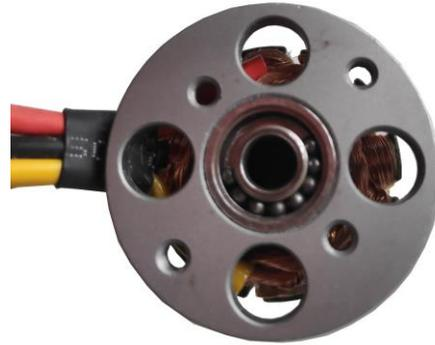
Figure 5. Motor with broken bearing cage.
