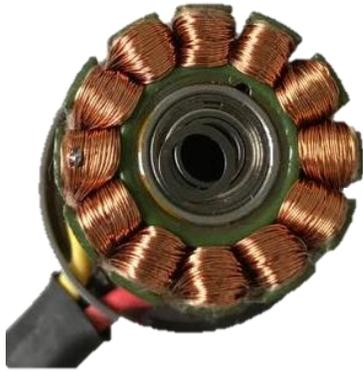
Figure 6. Manipulated stator with solder drop.
