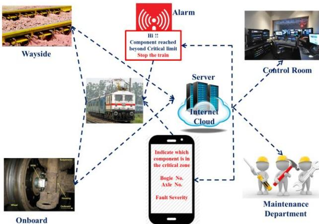
Figure 6. CBM architecture for railway
