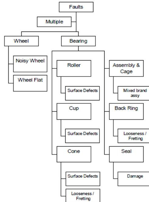
Figure 5. Bearing and wheel fault hierarchy (Southern, Rennison, and Kopke, 2004)
