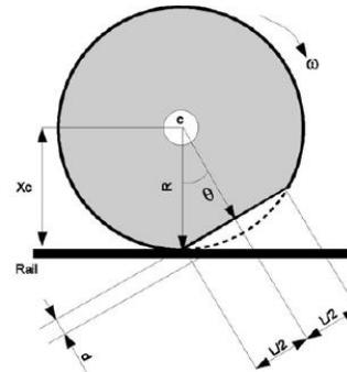
Figure 11. Simplified wheel flat measurement model (Brizuela et al., 2010)
