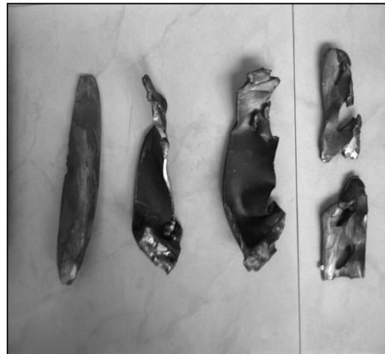
Figure 14. Rests of blades found in LP turbine after the trip.
