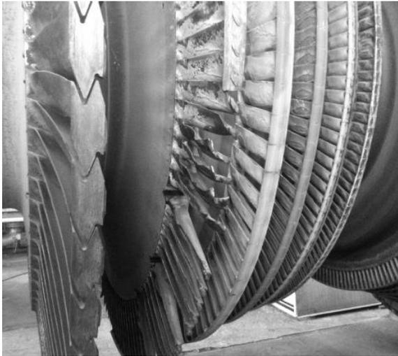
Figure 15. Rotor showing missing shrouds and 4 blades off, at positions: 7, 13, 19, 38 on stage 5 that has a total of 124 blades. On this side, 2 blades had been de-rooted.
