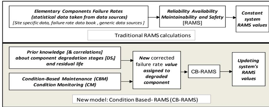
Figure 1. The CB-RAMS model versus traditional RAMS.
