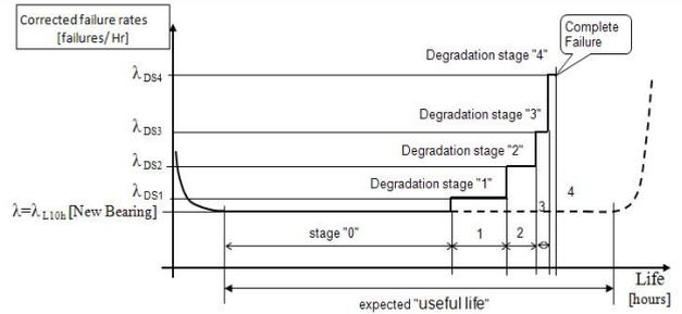
Figure 3. Theoretical expected useful life as predicted by regular RRMS, and shortened life after component wear is detected by CM and bearing is in degradation stages.
