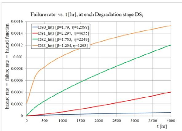
Figure 8. Failure rate calculation for each DS<sub>i</sub> versus time.
