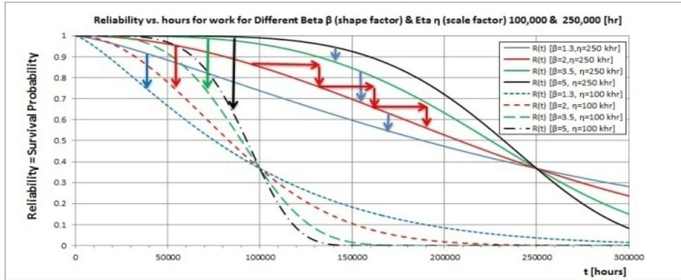
Figure 4. The influence of changes in Weibull parameters on the reliability. This graph is based on arbitrary generic parameters.
