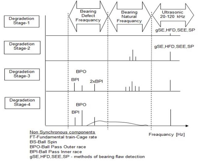
Figure 2. Typical Vibration spectrum for rolling bearing failure stages
