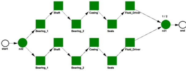
Figure 10: The MCS scheme for two-pump redundant system.
