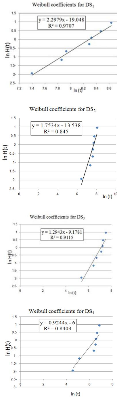
Figure 6. Weibull parameters  $\beta$  and  $\eta$  for each Degradation Stage  $DS_i$ .
