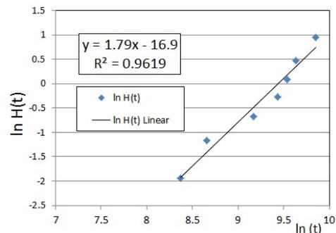
Figure 5. Graphical presentation of calculation of Weibull parameters, from new to Total Failure.
