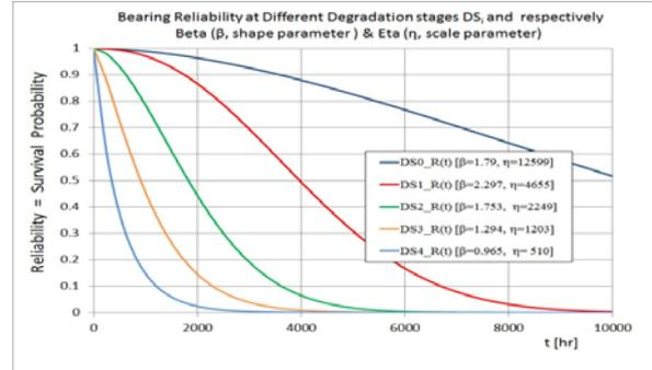
Figure 7. Bearing Reliability values as a function of  $DS_i$ .
