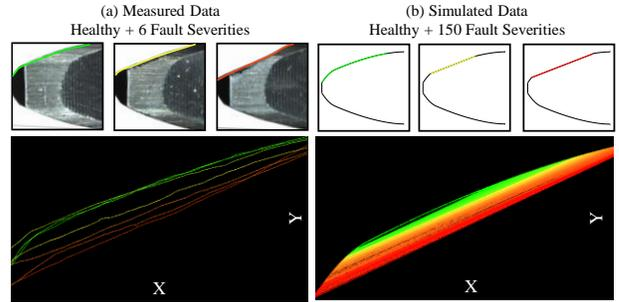
Figure 11. Tooth contours across severity of measured and simulated datasets in the case study.
