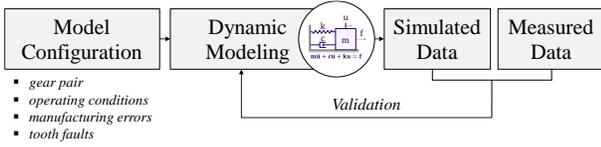
Figure 9. Block diagram of dynamic modeling and experimental validation.
