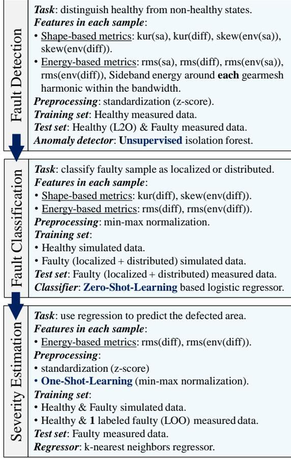
Figure 12. Schematic flow of the case study.
