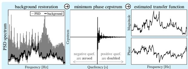
Figure 4. Illustration of the transfer function estimation.
