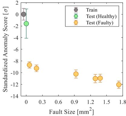
Figure 13. iForest anomaly scores vs. fault size.
