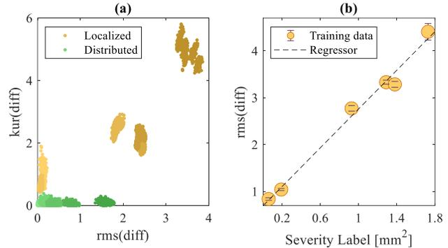
Figure 16. Benchmarking against fully supervised training: (a) fault classification shown by clear separation in normalized  $\text{rms}(\text{diff})$ - $\text{kur}(\text{diff})$  maps; (b) fault severity estimation illustrated by the  $\text{rms}(\text{diff})$  vs. severity label.
