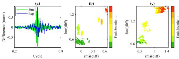
Figure 10. Validation of tooth destruction faults: (a) Comparison of normalized difference signals for the most severe fault; logarithmic maps of  $\text{kur}(\text{diff})$  vs.  $\text{rms}(\text{diff})$  across fault severity for (b) experiments and (c) simulations.
