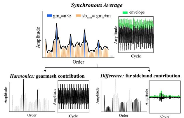
Figure 6. Scheme of synchronous average analysis, accompanied by a signal of a pitted gear.
