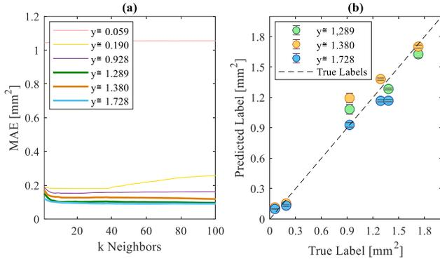
Figure 15. kNN-based severity estimator: (a) MAE vs.  $k$ -neighbors for different train severity labels; (b) Predicted vs. true labels for the three largest severity labels in training.
