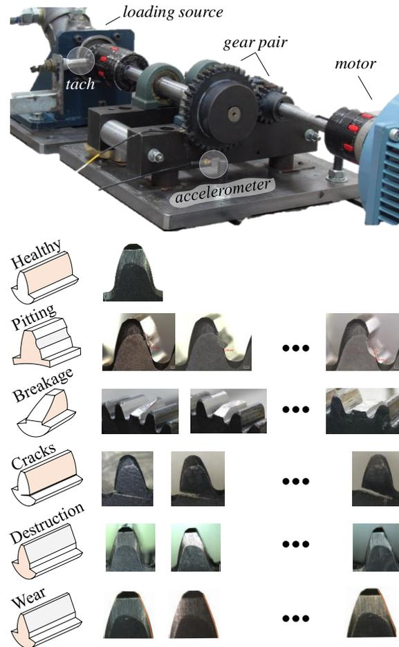
Figure 8. A typical gear test apparatus (top) and various controlled-degradation tests conducted (bottom).
