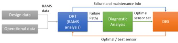
Figure 1: Framework for sensor optimization
