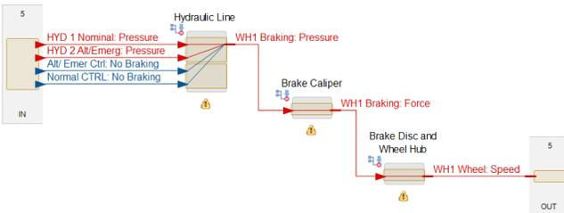
Figure 2 DRT of Wheel Brake Assembly 1
