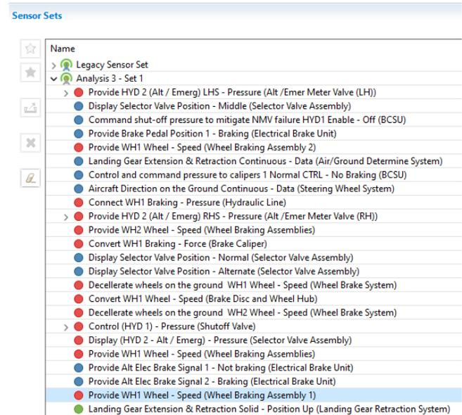
Figure 8: Identification of location for sensor deployment
