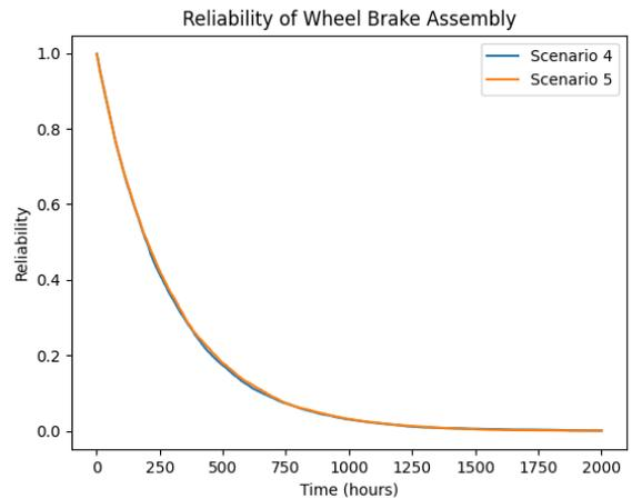
Figure 17: Change in system reliability by incorporating maintenance on sensor
