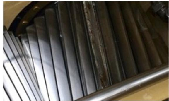
Figure 10. Damage High Speed Pinion
