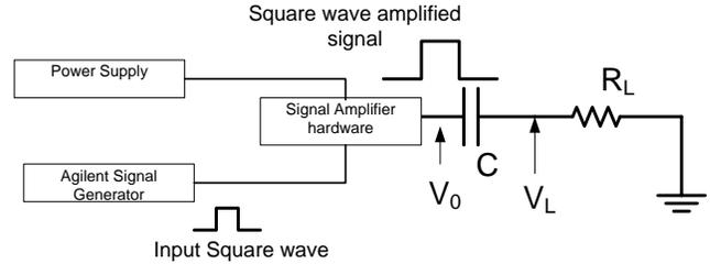
Figure 2. Block diagram of the experimental setup.
