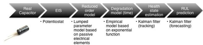
Figure 1. Model-based prognostics methodology for electrolytic capacitor.
