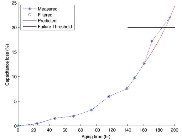
Figure 8. Remaining useful life prediction at time 149 (hr).
