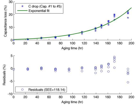
Figure 6. Estimation results for the empirical degradation model.
