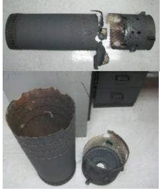
Figure 1. Broken liner as the result of cracks propagation
