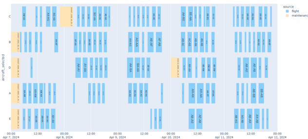
Figure 3. Flight (blue) and Maintenance (yellow) schedule resulting from deterministic optimization. Uncertainty is not considered in this framework.
