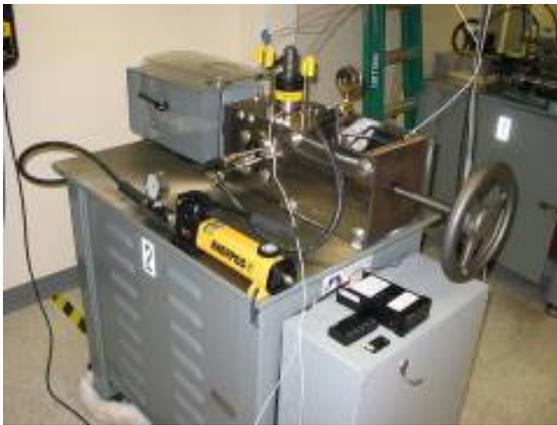
Figure 4: Subscale spall propagation test rig
