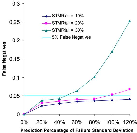
Figure 8. False negatives for varying prediction percentage of failure standard deviation by  $STMR_{fail}$ .
