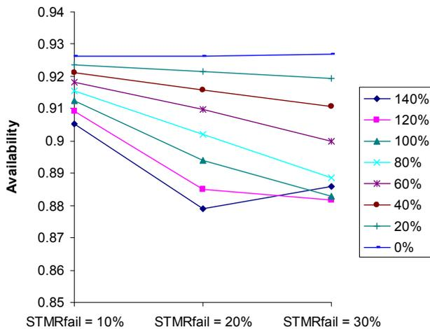
Figure 9. Availability for increasing  $STMR_{fail}$  by prediction percentage of failure standard deviation.
