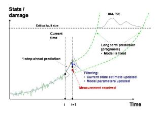
Figure 1: Concept of process model-based prognostics.
