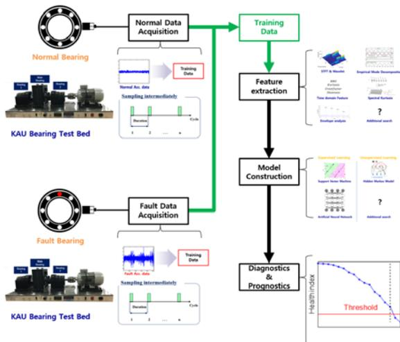
Figure 2. Bearing diagnostics flow chart
