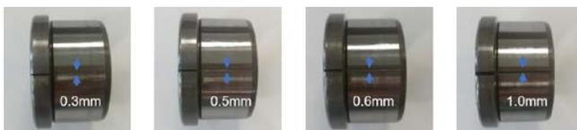
Figure 3. Bearings with imbedded fault
