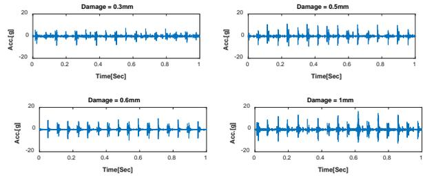
Figure 4. Vibration signal of bearings with different fault size
