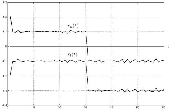
Figure 3. Behavior of the residuals  $r_u(t)$  and  $r_l(t)$  when the fault occurred.
