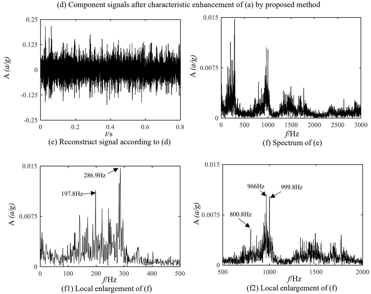
Fig 5. Bearing compound faults feature extraction - ITD+EWM
