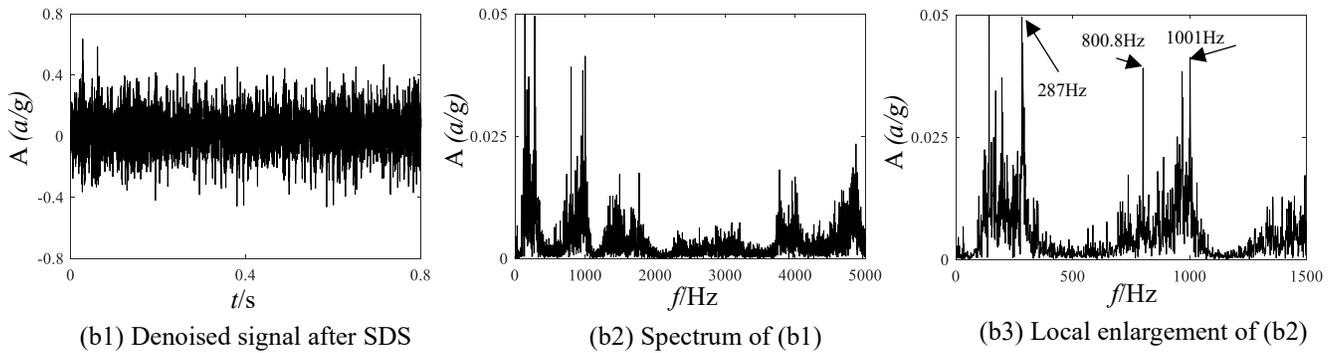
Fig 4. Compound faults feature extraction of bearing - SDS - inner ring + rolling element + outer ring faults
