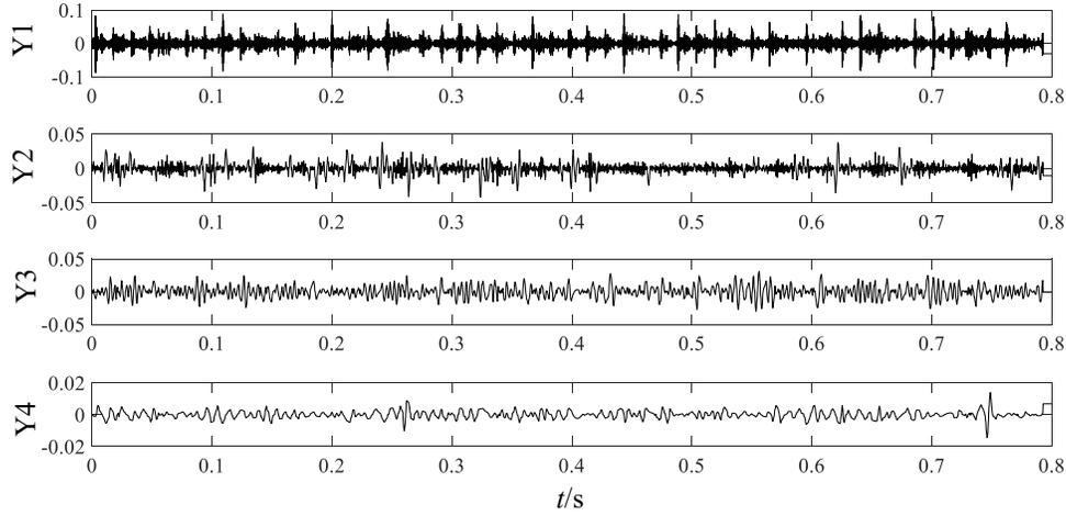
Fig 17. Component signals after characteristic enhancement of Fig 14 by proposed method
