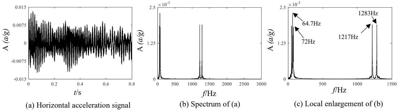
Fig 18. Time domain and frequency domain diagram of proposed method - outer ring + inner ring faults
