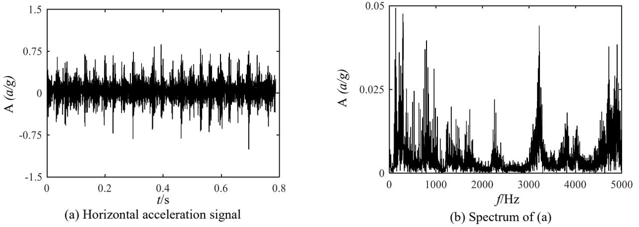
Fig 7. Time domain and frequency domain diagram of original signal
