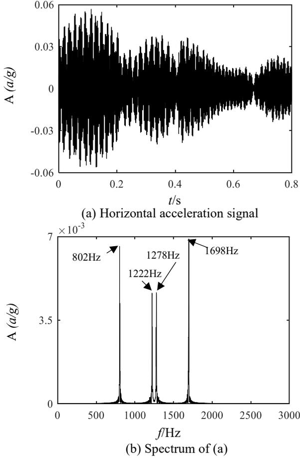
Fig 12. Time domain and frequency domain diagram of proposed method - inner ring + rolling element faults
