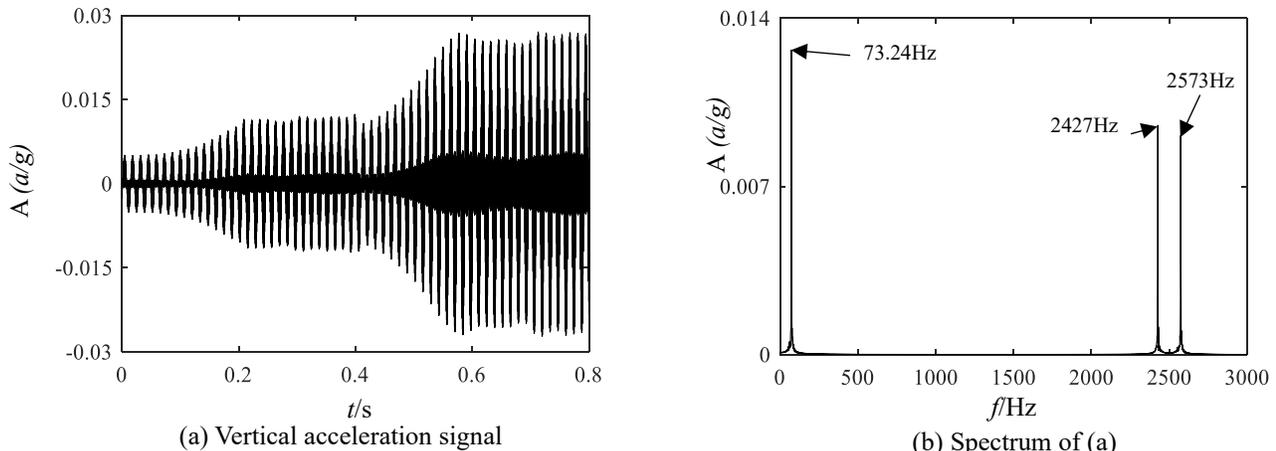
(a) Vertical acceleration signal (b) Spectrum of (a)
