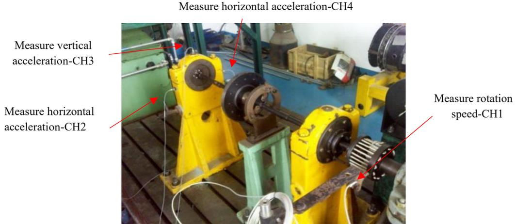
Fig 2. Aero-engine rotor-rolling bearing experimental rig
