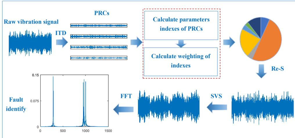
Fig 1. Method flow diagram. Note: ITD, intrinsic time scale decomposition; PRCs, proper rotation components; Re-s, reconstruct signal; SDS, singular value decomposition differential spectrum.
