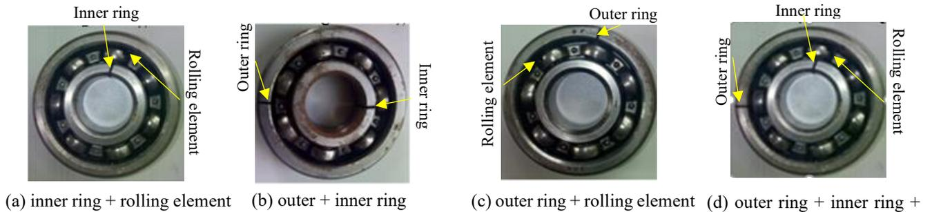
Fig 3. Compound faults of rolling bearing
